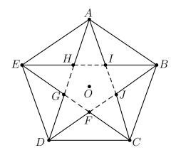
The sum of the internal angles in an n-gon is  $(n-2) \times 180^{\circ}$ . Hence each internal angle in a regular pentagon is  $(5-2)180/5 = 108^{\circ}$ .
